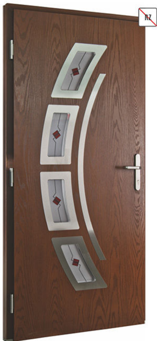
Model: DIPLOMAT 20 Color: Walnut Sash surface: RW Door handling: Left to outside Lock: 3-point strip lock lockable by door handle Hinges: adjustable 3D in color of fittings Stained glass: 3.1-24-T/D/T Variant of application: RN Fittings: handle Baron (F9)
